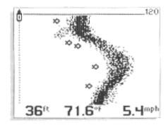
Experiment with the Wide Side transducer while operating it in a familiar area to learn how to maximize use of the information displayed. Remember that if you are using a trolling motor mount, the information displayed is controlled by the direction the trolling motor is pointing, not necessarily the direction the boat is traveling.
